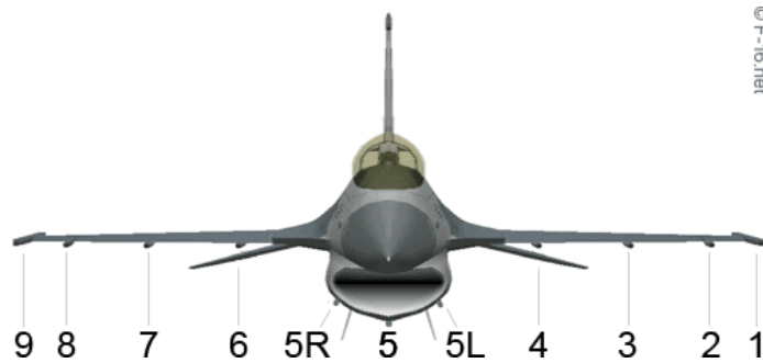
Figure 2 F-16 Pylon Loadout ( https://www.f-16.net/f-16_armament_article3.html )
